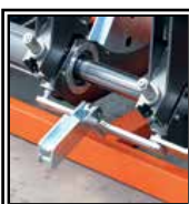
Detach device for heater
