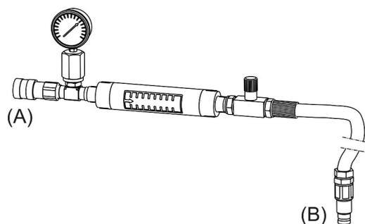
To set or check the hydraulic oil flow and the pressure relief valve we recommend using Chicago Pneumatic or similar test equipment.
