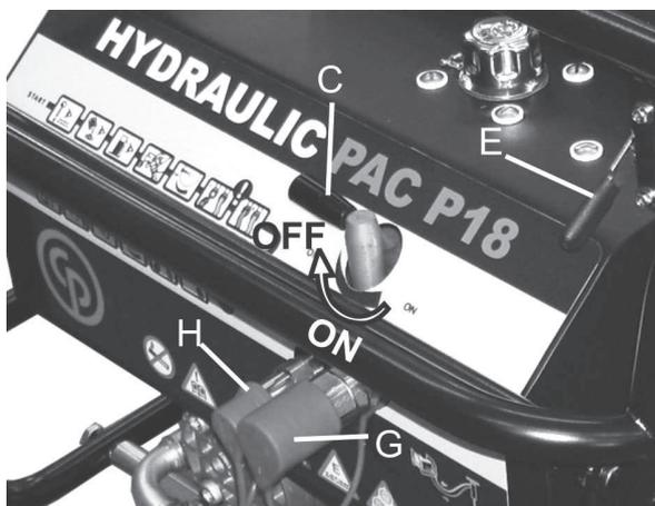
The by-pass valve (C) must be in the OFF position when starting and in the ON position when using the machine.
