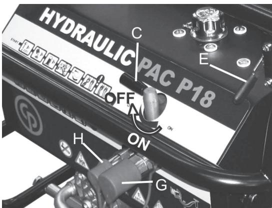
4. Turn the ignition key (D) clockwise. Let the ignition key go back to vertical position, when the engine starts.
