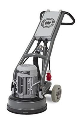
HTC Greyline™ 400 is a single headed three-phase grinder with an incredible removal rate. It is perfect for removal of floor coverings, molded joints and faults in the concrete from casting. The machine separates for easy transport.
