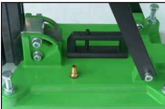
Connect the drill rig and the vacuum pump by means of a vacuum hose. Get the drill rig in the correct position and switch on the pump. Make sure, that all four levelling screws in the foot plate are turned back and that a low pressure of -0,8 bar is reached. By means of pressing the valve button in the handle the drill stand can be unburdened (vacuum is escaping) and can be readjusted.
