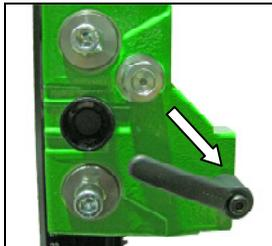
The machine holder has a special quick connection fixture for the machine. Thereby the prism on the gear box of the machine will be inserted from above in the dovetail fixture of the machine holder and braced firmly by the clamp hand gear on the side.
