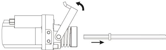
2. Insert the drill steel in the chuck.
