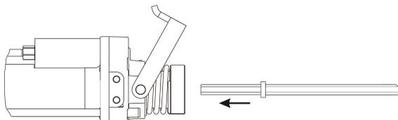
3. When the drill steel bottoms, push back the tool retainer to lock it.
