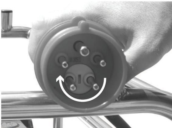
**NOTICE** Letting the motor rotate in the wrong direction for a long time can harm the pump.
