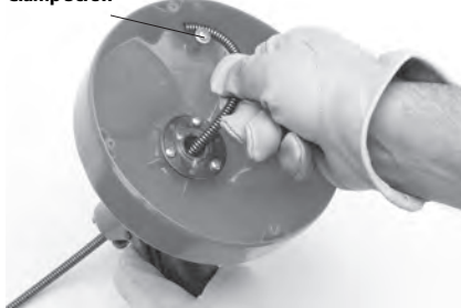
Figure 9 – Installing Cable End Into Holder
