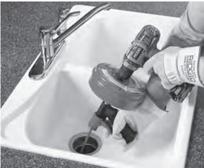
Figure 8A – Power-Spin Powered By Battery Drill
