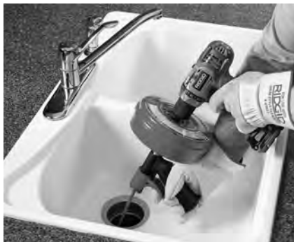
Figura 8A – Power-Spin Powered By Battery Drill
