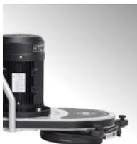
**The ability to adjust** the grinding head in both X- and Y-axis provide conditions for a perfect result when grinding. Furthermore, all settings are easily made without any need for special tools.
