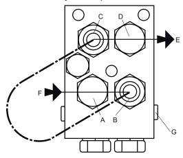
For clockwise rotation direction (when seeing the rock drill from above), connect a hose between the hydraulic ports A and C.
