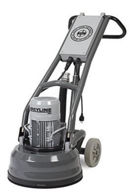
HTC Greyline™ 450 is a single-phase, planetary grinder with three grinding heads and a counter-rotating grinding wheel for a stabile grinding without lateral forces. It works equally well for concrete grinding and floor prep as it does for grinding/sanding of wooden floors. The machine separates for easy transport.
