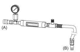
To set or check the hydraulic oil flow and the pressure relief valve we recommend using Chicago Pneumatic or similar test equipment.
