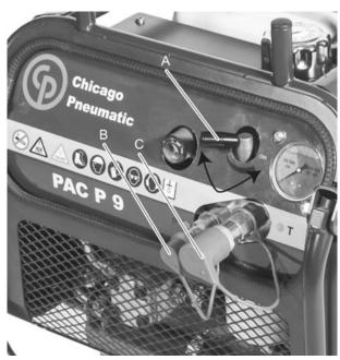
The by-pass valve (A) must be in the OFF position when starting and in the ON position when using the machine.
