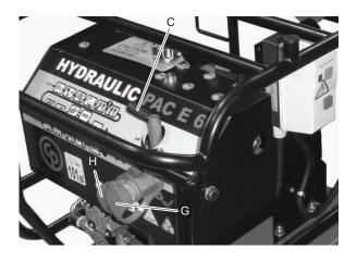
The by-pass valve (C) must be in the OFF position when starting and in the ON position when using the machine.
